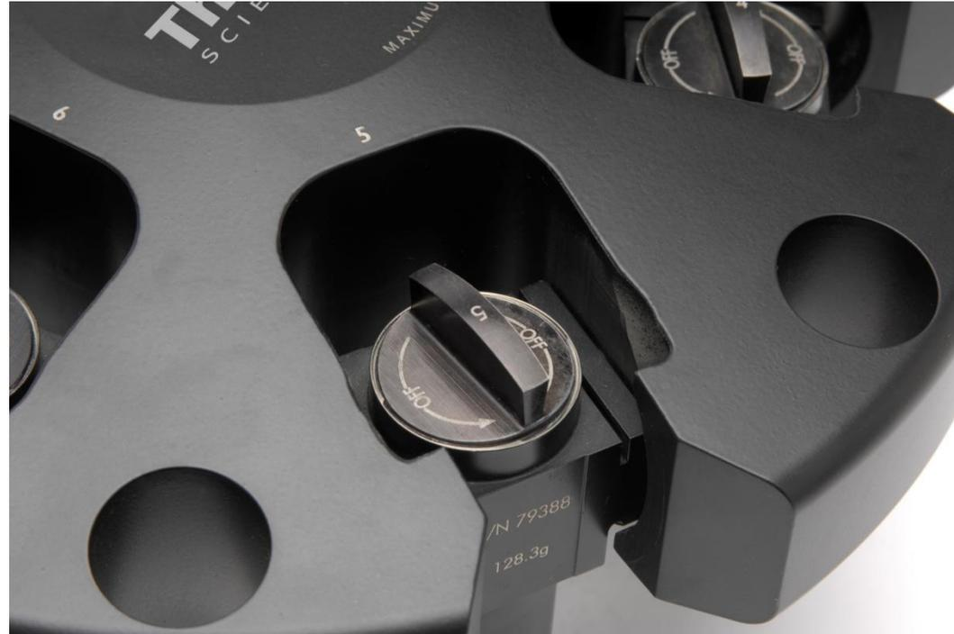
**For swinging bucket rotors, gently swing out each bucket to ensure a free easy motion. Always double check before pressing start**
