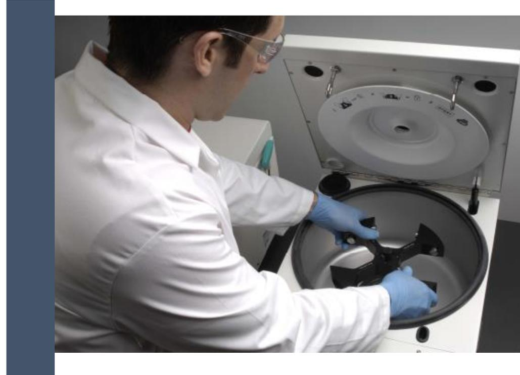
**Always double check that your rotor is locked down before pressing start !**
